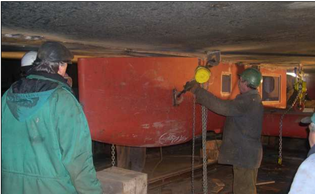
Figure 4 – “Nose” Fairing Installation
